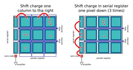
capacitance of the system is set by the SN: C=0.05pFightarrow 3 $\mu$ V/e
