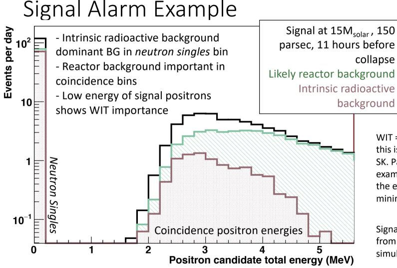
WIT = "Wide Intelligent Trigger" this is a software trigger system at SK. Parallel computers are used to examine every single hit, reducing the energy threshold to the minimum possible.
