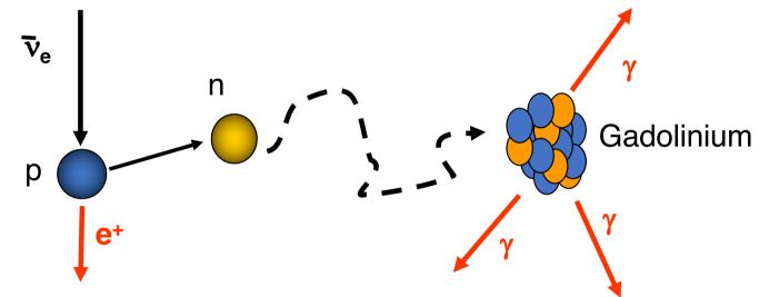
Gadolinium has a high **thermal neutron capture** cross section High energy of gamma ray cascade gives highly efficient neutron tagging
