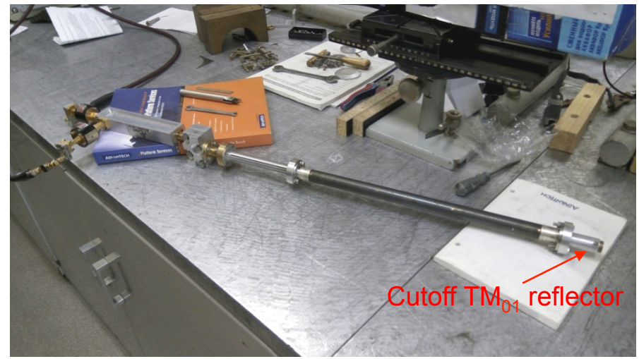
Reflection measurement scheme
