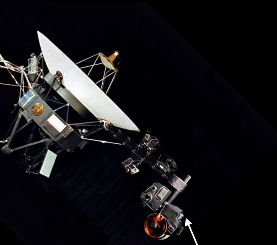
Plasma Science Experiment (PLS) Ions and Electrons: 10 eV – 5.9 keV
